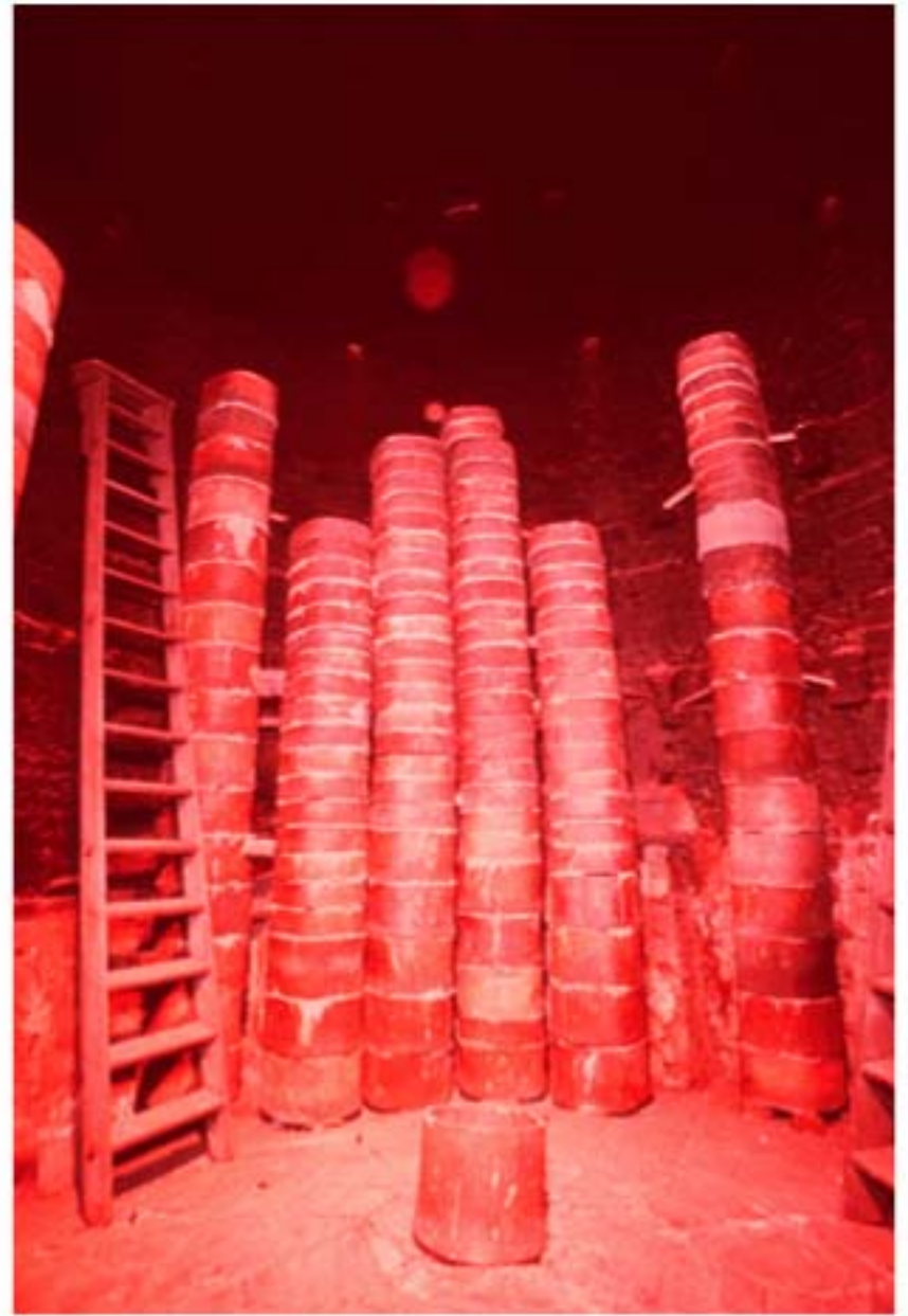
Interior view with saggers
